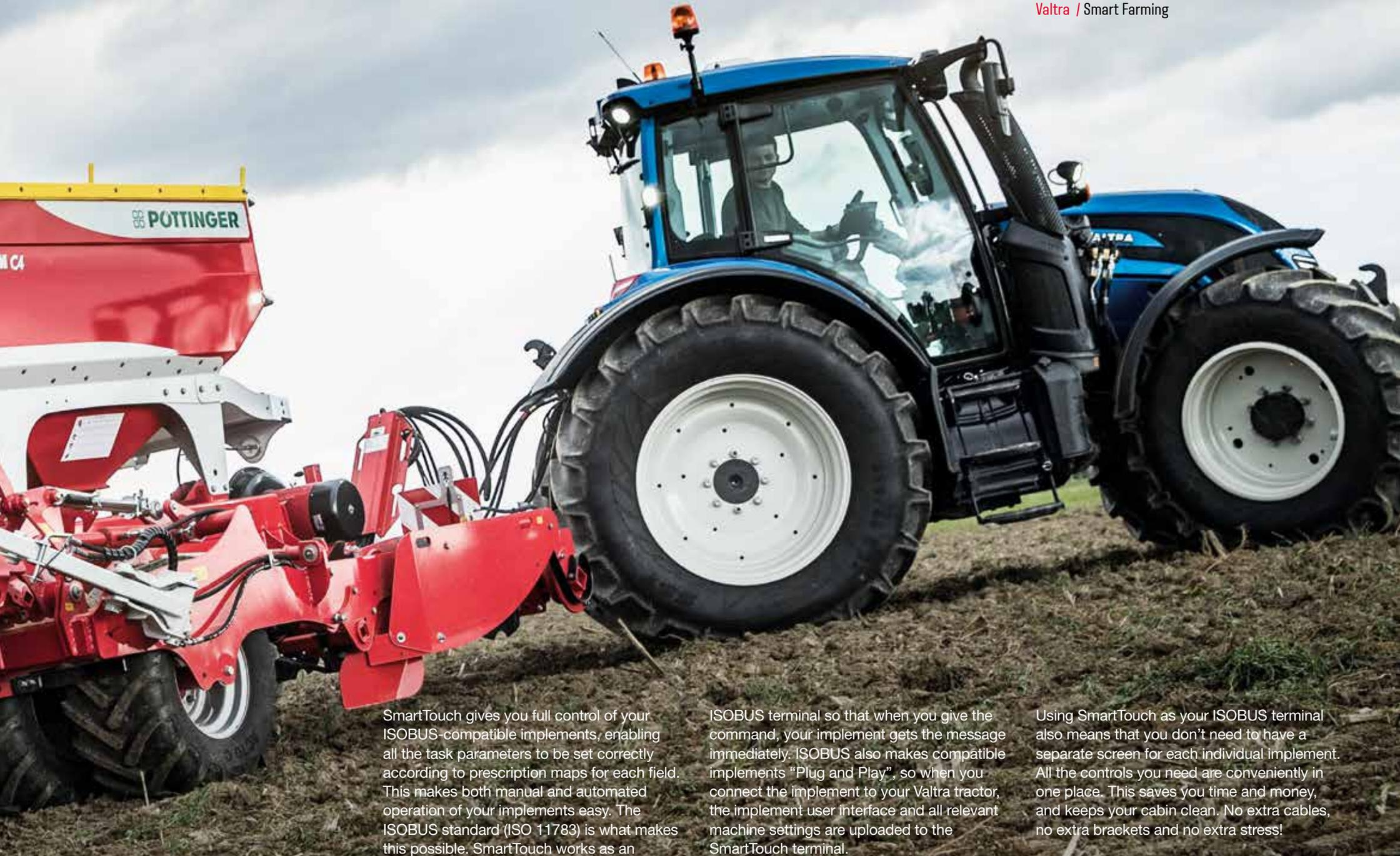
SmartTouch gives you full control of your ISOBUS-compatible implements, enabling all the task parameters to be set correctly according to prescription maps for each field. This makes both manual and automated operation of your implements easy. The ISOBUS standard (ISO 11783) is what makes this possible. SmartTouch works as an
