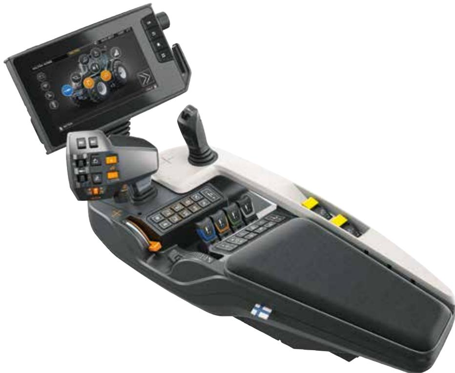
Valtra SmartTouch brings easy living to your fingertips – literally. It combines a 9" touchscreen with clearly arranged buttons, a multifunction lever, a hydraulics joystick and a comfortable armrest. It's simple, well laid-out, and really easy to use and it gives you complete control of all your smart farming functions.
